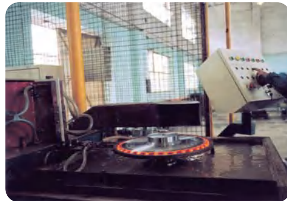
Special Heat Treatment to Increase the Hardness and Wear Resistance of the Teeth
